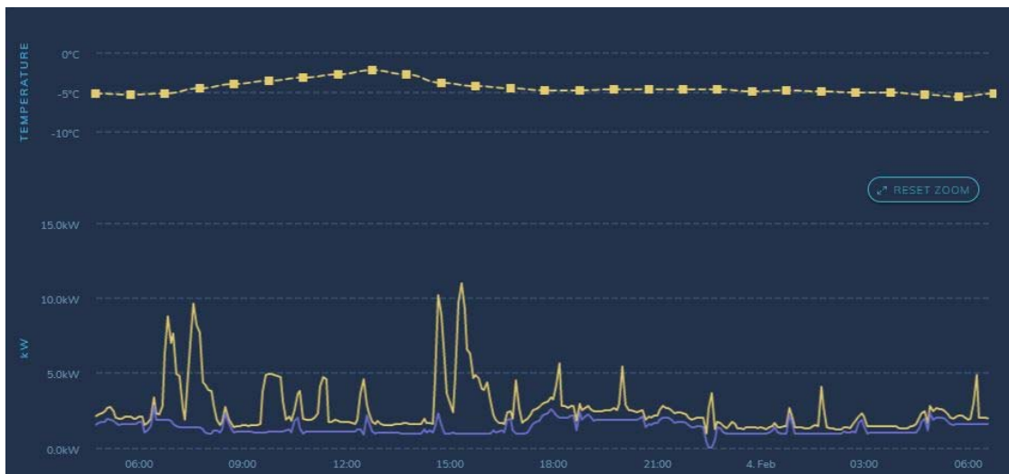
Figure 18: Example DHP with Potential Defrost Mode Power Surges
