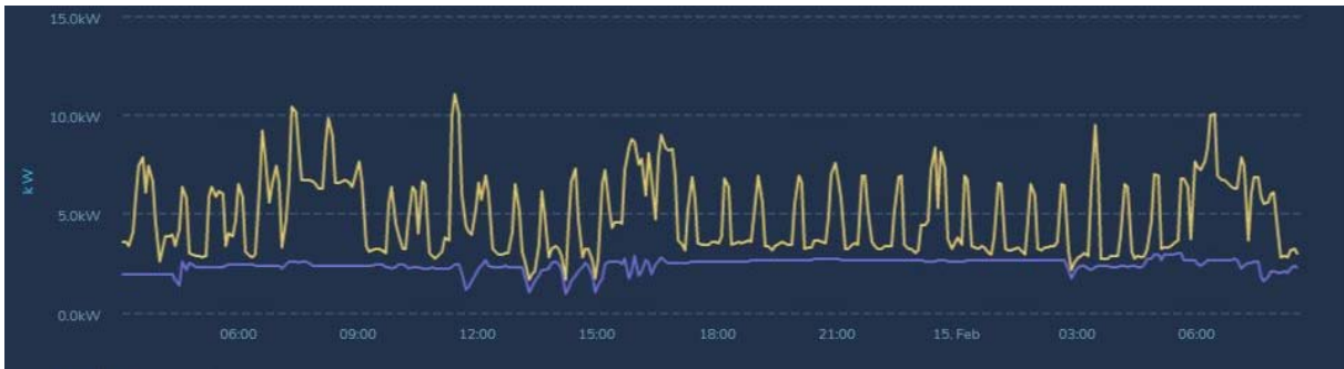
Figure 17: Example DHP with Rapid Oscillations
